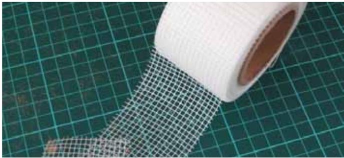
However, you need to cut this into a strip to the width and length you need before pressing it onto the felt. If you try to lift it away from the felt once it is allowed to stick, the felt will easily tear away spoiling the look — and the adhesion!
